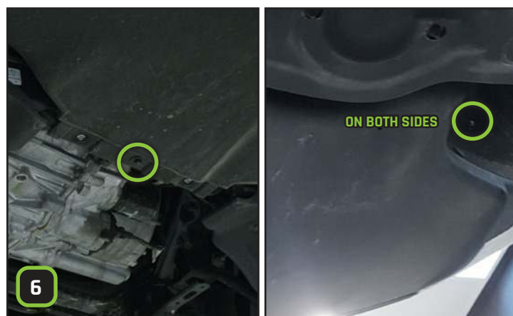
Undo the bolt in middle and two bolts marked in the backside of the rear wheel well covers.
