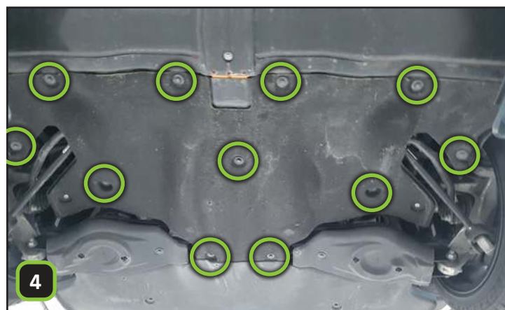
Undo the marked bolts (11x) and remove the cover panel behind the rear wheels.
