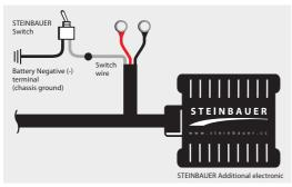
Connect the grey wire of the switch to the Switch wire (grey wire of the STEINBAUER Additional electronic). Connect the black wire of the switch to the battery Negative (-) terminal (chassis ground).
