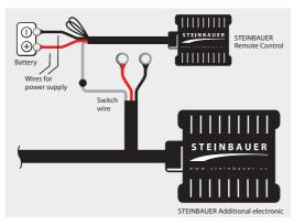
Connect the red wire to the battery Positive (+) terminal, black wire to the battery Negative (-) terminal. Connect the grey wire of the remote control to the Switch wire (grey wire of the STEINBAUER Additional electronic).
