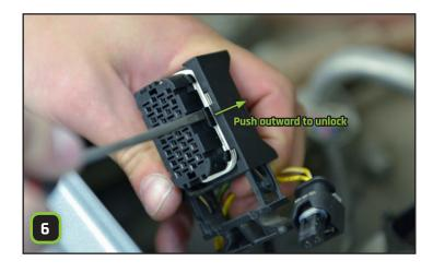
Unlock the pins by **disengaging the safety flaps** on the connector.
