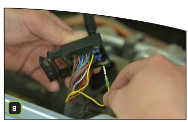
**Pull out the two wires** completely. The wires are colored **yellow (9)** and **yellow-white (8)**.
