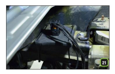
**Secure the STEINBAUER EV Module** to the chassis then **connect the harness**.
