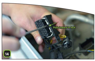
**Engage the safety flaps** using a flathead screwdriver.
