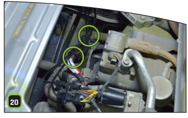
**Secure the wiring harness to the coolant pipe** behind the motor.
