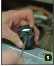
**Unplug the connector** and **remove the plastic cover** using a flathead screwdriver.
