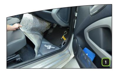
Access the **12V battery** by lifting the passenger footwell carpet and removing the styrene panel.
