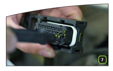
Push out **PIN8** & **PIN9** from the connector using a **small pin tool**.
