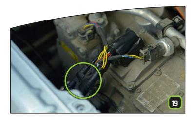
**Secure the elements of the wiring** together behind the connector using **zip-ties**.
