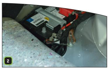
**Disconnect the 12V battery** before proceeding with the installation!
