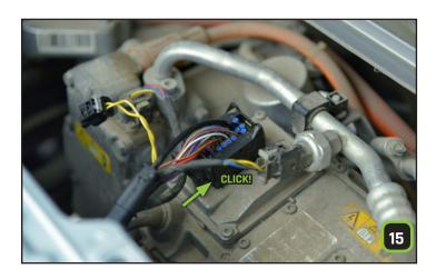
Reconnect the motor connector and lock it.
