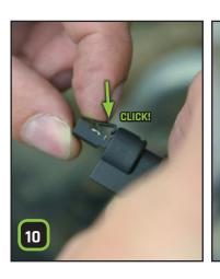
**Lock the pins** by pushing the safety flap on the end of the connector down **until it clicks**.
