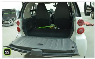
**Refit the metal engine cover** and fold the trunk carpet back down.
