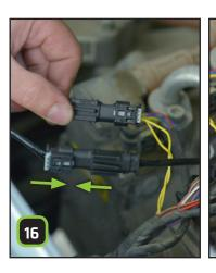
**Connect** the other end of the **STEINBAUER** harness to the other 2-pin connector.
