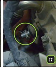
Remove the plastic cap & **connect the red wire** (+) **under the 10mm bolt**. Then refit the cap.
