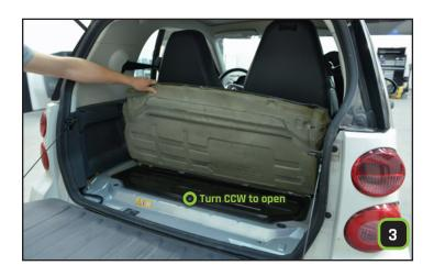
Fold up the **trunk carpeting** and remove the **metal plate** covering the engine compartment.
