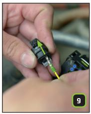
Pin the two wires into the **supplied connector**. **PIN 1 - yellow/white** & **PIN2 - yellow**.
