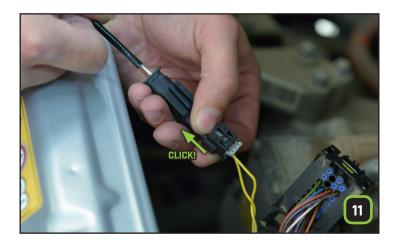
Connect the **2-pin connector** to the **female end of the STEINBAUER harness**.
