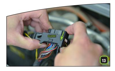
**Secure the pins** by pushing on the bottom of the connector **until you hear a click**.
