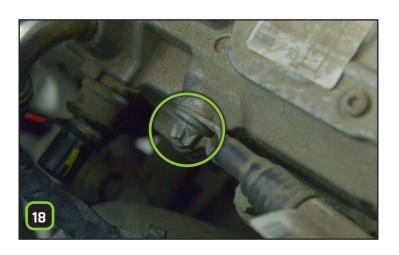
Connect the black wire (-) under the T13 Torx bolt on rear side of the motor.
