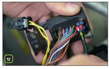
Pin the ends of the **supplied short cable** into the connector. **PIN8 - brown** & **PIN9 - white**.
