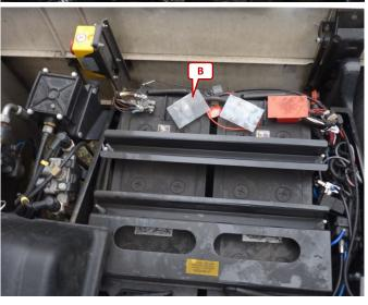
Connect the power supply to the battery (B). Connect the module to the adapter cable. Move the adapter cable not in parallel with injection pipelines or ABS-control device connecting leads. Keep to very big distances. Fix the cable harness with cable ties. The module should be obstructed possibly against warmth and splash water protected. Check all connections again and reassemble the vehicle in reverse order.
