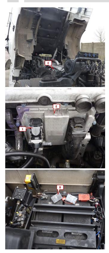
Mounting position engine control unit (E)
