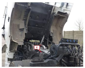
Mounting position engine control unit (E)
