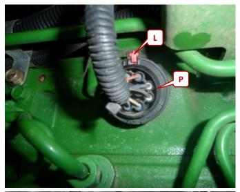
Localise then the 10 pin round plug (P). To unlock the connection you have to pull out the red pin (L). Turn the plug counter-clockwise to open it. Connect the adapter to the original plug.
