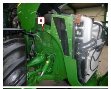
Open the engine hood. Localise the rail pressure bar (B).
