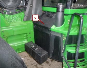
Localise the vehicle battery . Connect the  $\pm 12V$  clamp to the positive pole from the vehicle battery. Connect the ground clamp to the ground from the vehicle body or to the negative pole.
