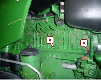
The rail pressure sensor (R) is in front off the rail pressure bar.
