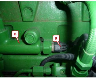
Disconnect the original rail pressure plug and connect the adapter cable with the rail pressure sensor. Connect the original rail pressure plug to the adapter cable.
