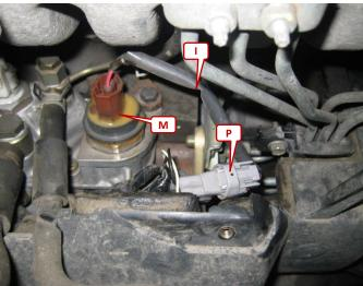
Localise the plug from the cable (I) which goes up from the magnetic valve (M). Open the 2pole plug (P). Connect the right adapter cable between the connector plugs.
