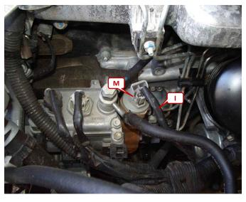
Use only the cable (I) which is connected on the magnetic valve (M).
