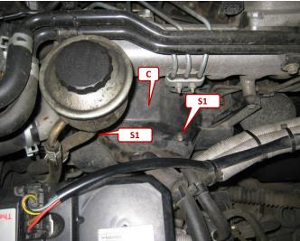
Solve the both screws (S1 and S2)from the injection pump cover (C).
