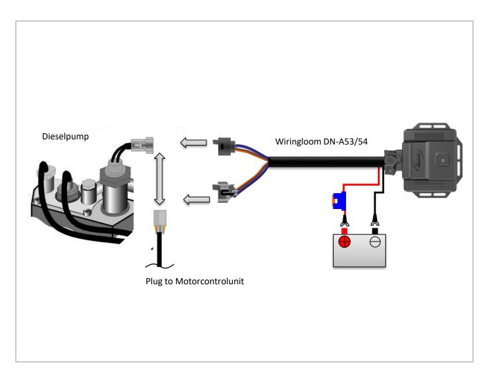
Localise the 2 pole plug from the cable which goes up from the magnetic valve. Open the 2pole plug. There are two different kinds of connection. You can see the difference in the form of the connector plugs. For this reason we deliver two different adapter cables (DN A53 and DN A54).
