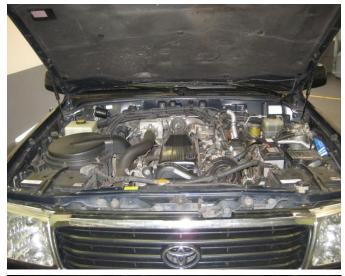
Switch the ignition off. Wait, until all electric power consumers are witched off. Open the engine hood.
