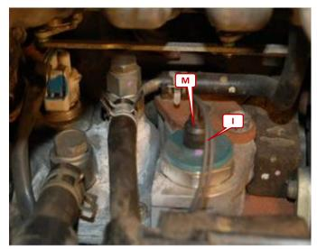
Use only the cable (I) which is connected on the magnetic valve (M).
