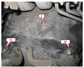
Solve the both screws (S1 and S2) and remove the cover (C).
