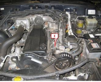
The injection pump (E) is on the right side from the engine.
