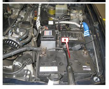
Connect the power supply at the vehicle battery (B). Move the cable if possibly splash water protected and avoid attaching in hot engine parts. Connect the module to the adapter cable. Now fit the cover back on. The vehicle is ready for a test drive. To restore the standard state, you must remove only the module. The adapter cable can remain connected.
