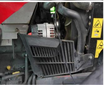
Connect the power supply of the adapter cable to the alternator of the tractor. The red wire has to be connected to the plus pole (red) of the alternator. The black wire to vehicle body ground.
