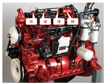
Locate the four 2-pin injector connections.
