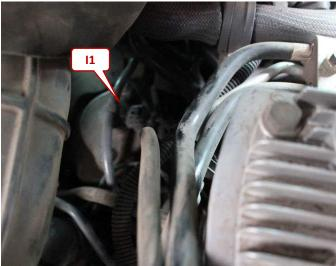
Disconnect the 2-pin injector connector 1 and connect the 2-pin plug of the adapter cable with the original connections.
