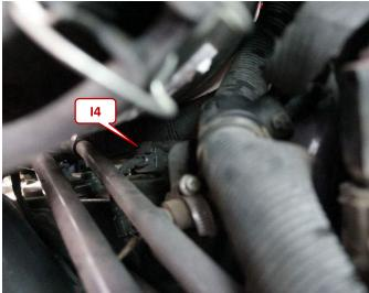
Disconnect the 2-pin injector connector 4 and connect the 2-pin plug of the adapter cable with the original connections.
