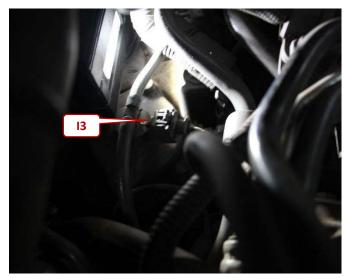
Disconnect the 2-pin injector connector 3 and connect the 2-pin plug of the adapter cable with the original connections.
