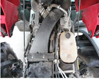
Disassemble the front part of the air filter box.
