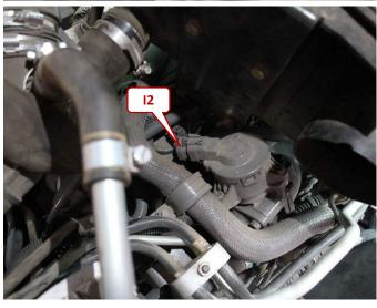
Disconnect the 2-pin injector connector 2 and connect the 2-pin plug of the adapter cable with the original connections.
