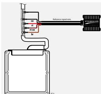
Connection Plugging in, simple method Open Locked Cable clip Cable clip
