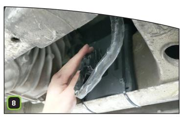
**Secure the STEINBAUER EV Module** to the chassis then **connect & lock** the wiring harness.
