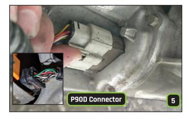
Unplug the connector on the **right-hand side** of the rear electric motor.
