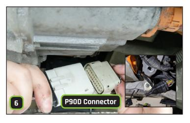
Plug the **male end** of the STEINBAUER wiring harness **into the original motor wiring.**
