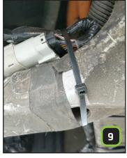
**Secure the wiring harness to the chassis** using zip-ties. Keep it away from the rear axle!
