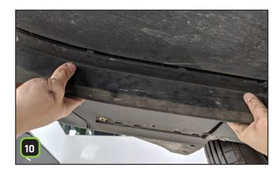
Refit the **rear splash guard and the diffusers.** Make sure to **use correct torque on the bolts.**
