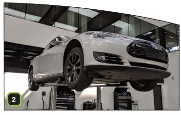
**Lift up** the vehicle. Tools you will need: **10mm socket, Torx T30, flathead screwdriver.**
