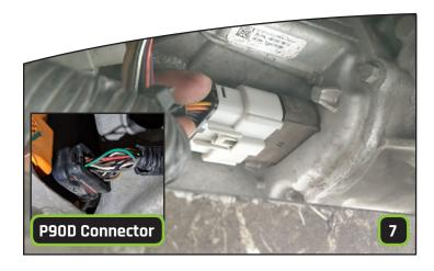
Plug the **female end** of the STEINBAUER harness **into the connector on the motor.**
