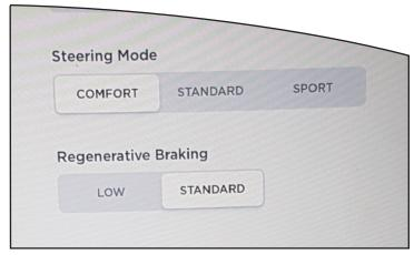
You can **disable the EV PowerModule** by setting **Regenerative Braking** to **LOW**.
