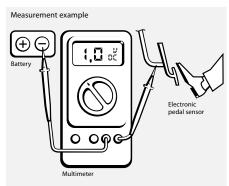
Measure the voltage with a multimeter on the plug-in
