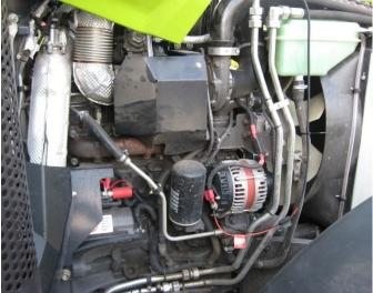
Lay the adapter cable to the other side in direction alternator.
