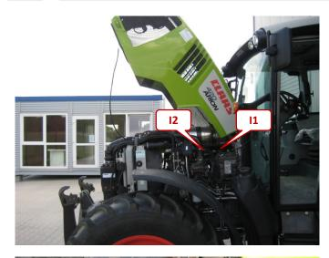
Open the engine hood. Localise the right side of the engine see in driving direction. Localise the both 4-pin injector plugs (11) and (12).
