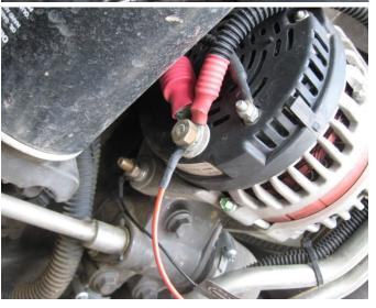
Connect the power supply + 12 V clamp to the positive pole from the generator. Connect the ground clamp to the ground connection from the alternator or to the vehicle body. Fix the cable harness with cable ties. Connect the module to the adapter cable. Check all connections again and reassemble the vehicle in reverse order.
