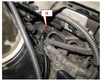
Connect the adapter with the mark (2) in between the original connection (12).
