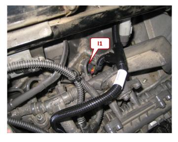
Connect the adapter with the mark (1) in between the original connection (11).
