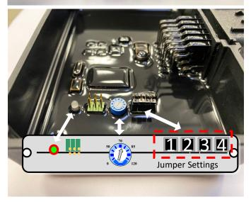
To change the basic settings of the VPC module, solve the 4 Torx screws (**T1** - **T4**) on the back side.
