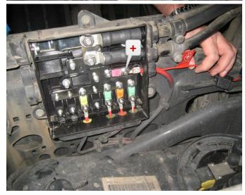
Connect the adapter cable in between each connection. The plugs fit only in one position.
