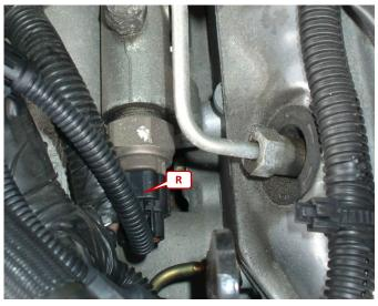
To disconnect the rail pressure plug press the locking lever. Connect the rail pressure adapter in between the both connections.
