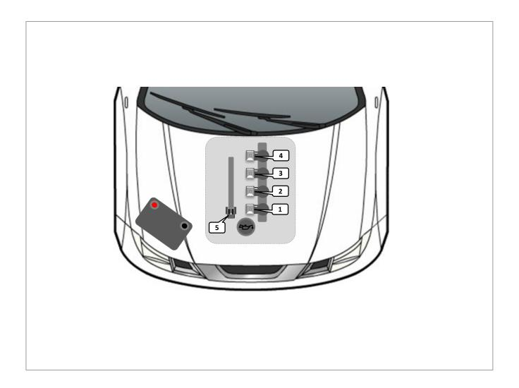
1 Injector Connector (2 pin)
