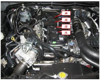
Localise the four injectors (J1–J4). Open the four 2-pole injector plugs. Connect the adapter cable to the original male plugs. Connect the original female plugs to the adapter cable. Start connecting from injector 1 to injector 4. On which side you start is not relevant. Don't connect it cross over.
