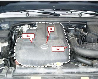
To remove the engine cover (D) solve the both screws (S1 -S2).
