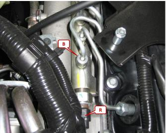
The rail pressure sensor (R) is in front of the common rail bar (B).
