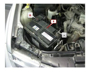
Connect the power supply at the vehicle battery (B). (+ to the positive pole and - to the negative pole). Connect the module with the adapter cable plug. Move the adapter cable not in parallel with injection pipelines or ABS-control device connecting leads. Keep to very big distances. Fix the cable harness with cable ties.
