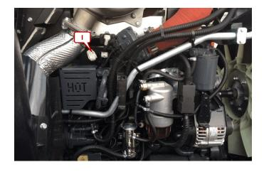
Localise the right side of the engine see in driving direction. Localise the 10-pin injector plug (I). Open the injector plug. Connect the adapter cable in between these connection.
