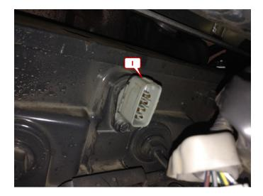
Connect the power supply to the vehicle battery. You can alternatively connect the + 12 V clamp to the positive pole from the generator. Connect the ground clamp to the ground from the vehicle body. Fix the cable harness with cable ties. Connect the module to the adapter cable. Check all connections again and reassemble the vehicle in reverse order.
