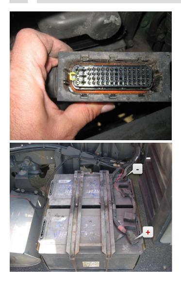
Note the position of the plug. Connect the adapter cable in between this connection. It fits only in one position. Close the plug by pushing the yellow locking lever to the right.
