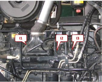
Localise the three 4-pin injector connectors (I1-I3). Disconnect the original injector plug and connect the adapter cable with the original injector. Note the sequence. (I1  $\rightarrow$  Cooler / I2  $\rightarrow$  concentrically / I3  $\rightarrow$  driver cabin) Connect then the original plug to the adapter cable.
